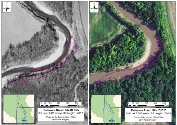
Figure 2: 2002 FSA & 2015 NAIP of a Streambank Erosion Site on the Delaware River
