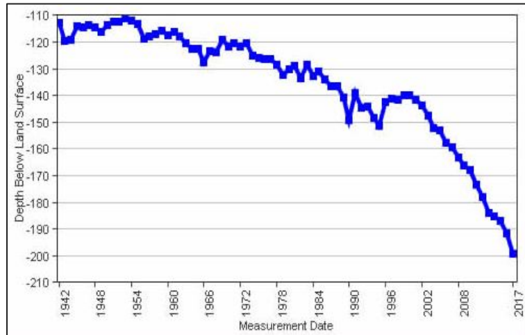
Figure 7: Hydrograph showing the decline of the Ogallala Aquifer through time, with well measurements near Garden City in Finney County
