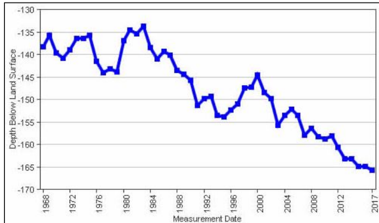
Figure 9: Hydrograph showing the decline of the Ogallala Aquifer through time, with well measurements near Dodge City in Ford County
